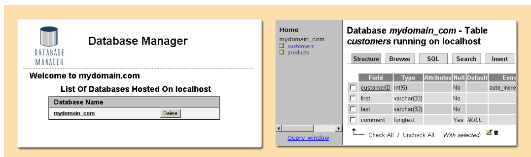
Figure 1: The Main interface (left) and phpMyAdmin window (right) of the Database Manager GUI.
